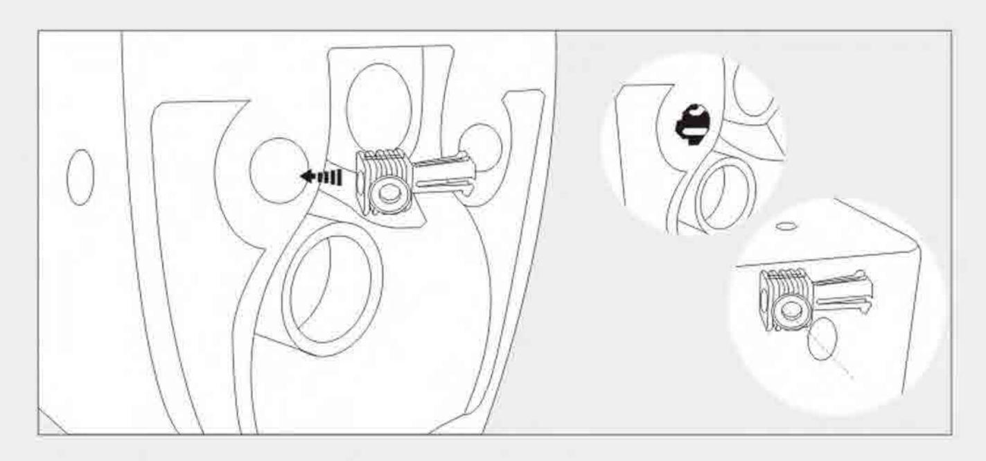
● 3. 将C套入挂便器的安装孔上。 Put Part C into the installing hole on the pan;
