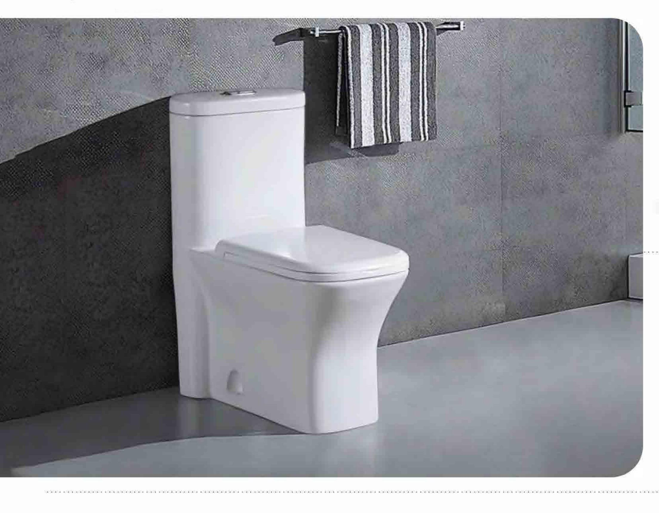
Washdown one-piece toilet Size:700x390x680 mm P-trap,180mm roughing-in S-trap,300mm roughing-in
