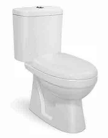
Washdown two-piece toilet Size:600x350x785 mm P-trap,180mm roughing-in S-trap,250mm roughing-in
