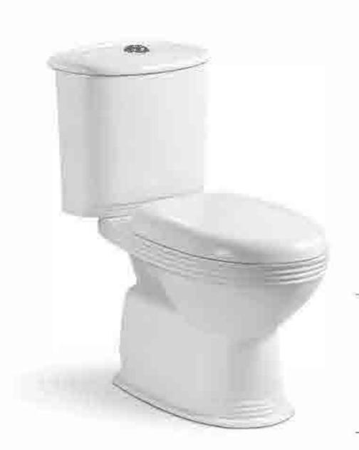
Washdown two-piece toilet Size:680x410x790 mm P-trap, 180mm roughing-in S-trap, 250mm roughing-in
