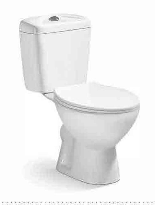
Washdown two-piece toilet Size:680x380x750 mm P-trap,180mm roughing-in S-trap,200mm roughing-in
