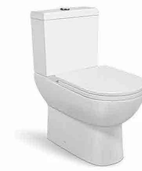
Washdown two-piece toilet Size:640x360x780 mm P-trap,180mm roughing-in S-trap, 150/250mm roughing-in
