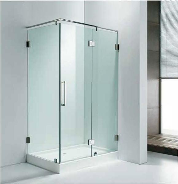
FC-516 Size : 800x1200x2000mm 900x1200x2000mm 1) 304# stainless steel rail/hings/handle 2) Clear color tempered glass in 8mm 3) One open door, Two fixed glass 4) With acrylic shower tray
